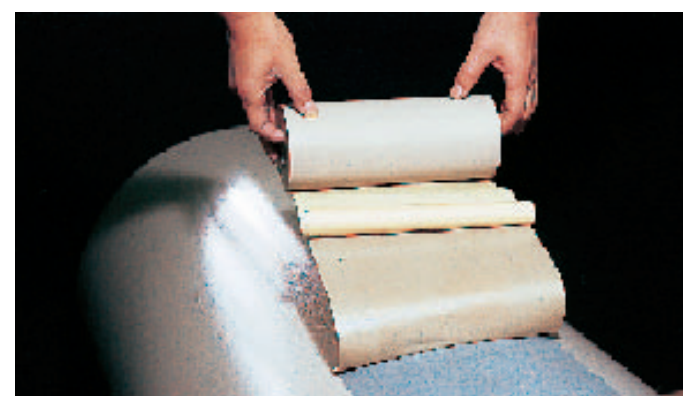
Release paper, coming with this type of adhesive tapes, makes it easier to cover large diameter rolls with the tapes.
